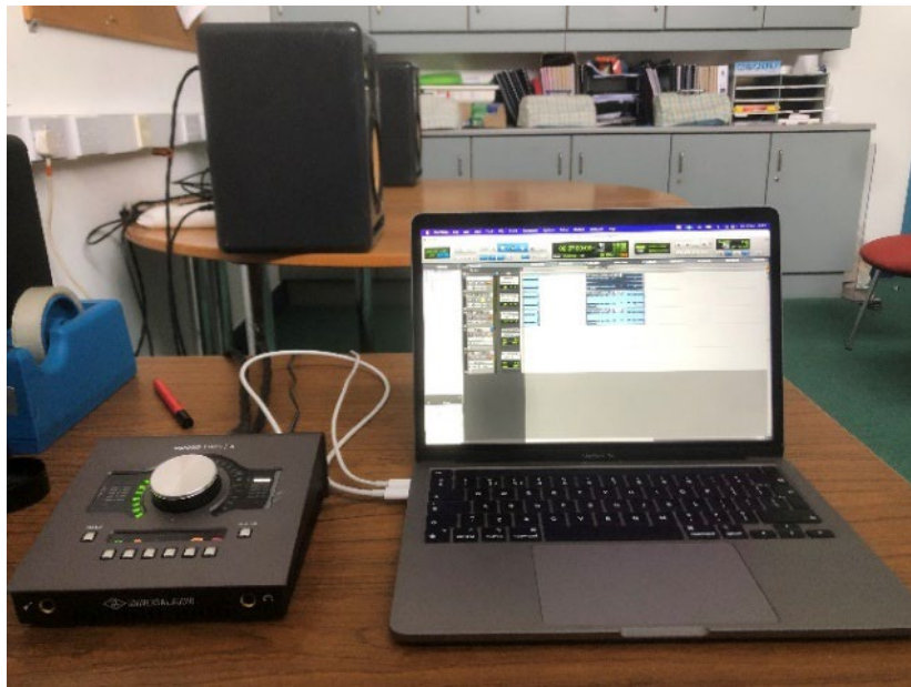
Image 5: Playback system - Pro Tools, MacBook Pro, UA Apollo Twin audio interface.
